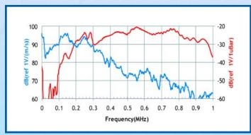
Frequency response of the WDI. Calibration based on ASTM E1106; Calibration based on ASTM E976.
